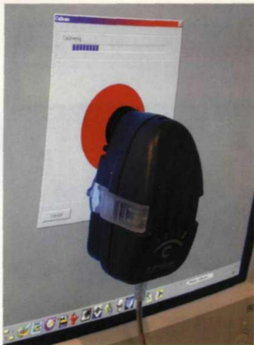
The X-rite Monitor Optimizer with software program is used to create monitor profiles.
